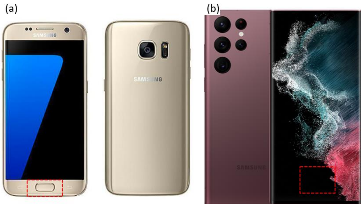
Figure 2.4 - Image showing the devices fingerprint sensor with (a) a thin button (CeX, 2022) and (b) no button highlighted (O2, 2022) with red boxes
