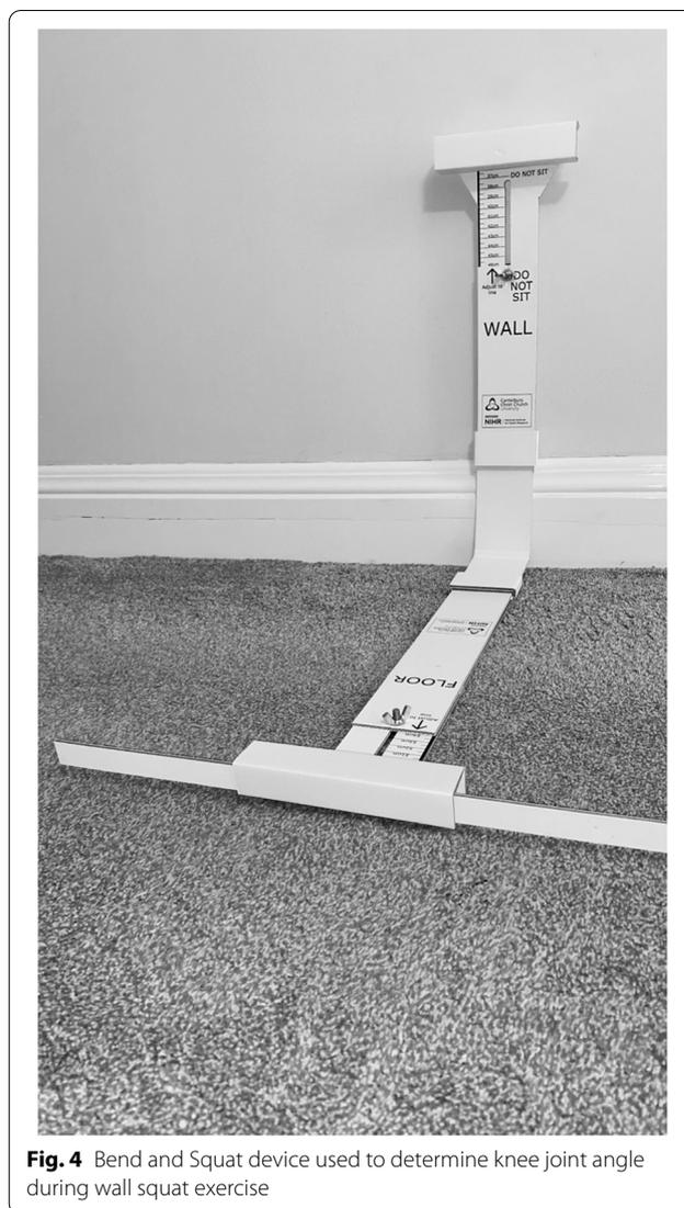
**Fig. 4** Bend and Squat device used to determine knee joint angle during wall squat exercise
