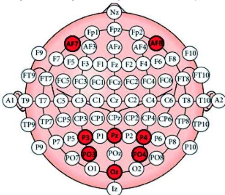
Front electrodes (AF7 and AF8) are used for the detection of three EMG signals; blink, left wink and right wink. After extensive testing, it was found that these two electrodes gave the most noticeable and distinctly individual signals, with minimal noise interference. The remaining six electrodes (Pz, P3, P4, PO3, PO4 and Oz) are located equidistantly around the visual cortex of the brain, so as to be able to pick up visually evoked potentials triggered by the P300 GUI.
