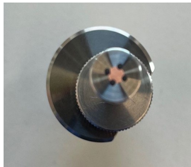
Figure 2 Cu and Al Standard on the mount for SEM-EDX Analysis
