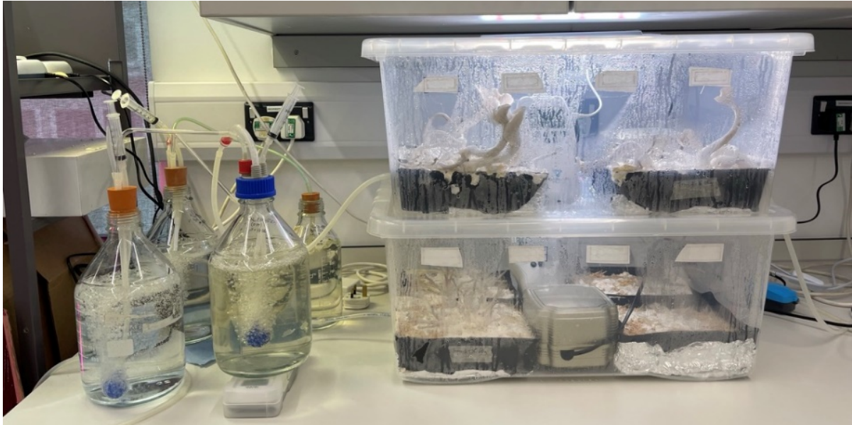
Figure 2.2 Experimental setup for carbon dioxide harvesting from mushroom production to generate inorganic carbon media for microalgae cultivation.
