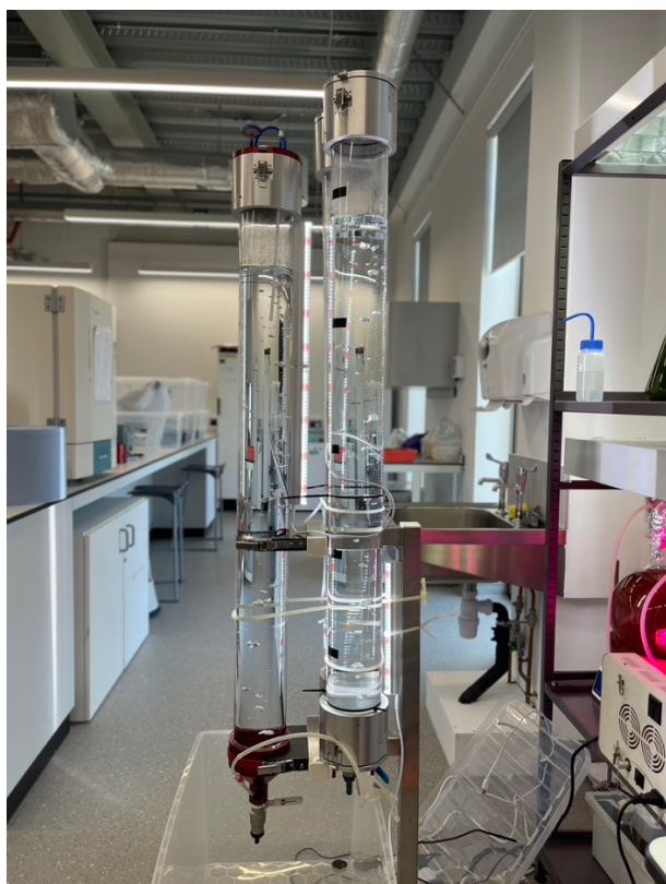
Figure 2.3 Bubble column photobioreactor scale-up with bicarbonate media generated from mushroom production before inoculation.
