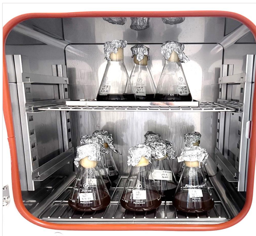
Figure 2.2 - Fermentation set up for wastewater treatment in a stationary incubator.
