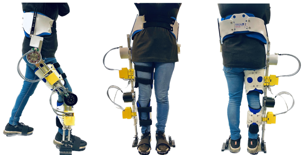
Figure 1. The prototyped SLE with two actuated joints at the hip and knee from side, front, and back perspectives.
