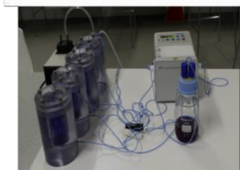
c) Perfusion bioreactors set up for studying fluid flow effect on osteogenesis
