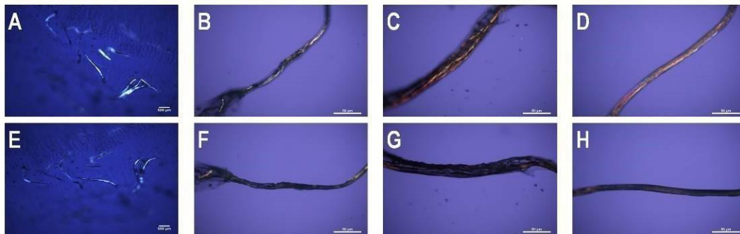
Figure 5 - (A, B, C, D) Polarised microscopy imaging of randomly aligned collagen films and electrochemically aligned 2, 4 and 8 mg / ml collagen fibres respectively (45° inclination); (E, F, G, H) – Polarised microscopy imaging of randomly aligned collagen films, electrochemically aligned 2, 4 and 8 mg / ml collagen fibres respectively (0° inclination).
