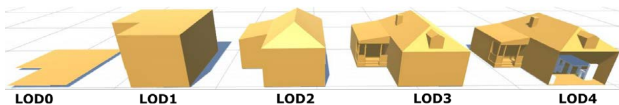
Figure 1. Level of detail (LOD) for buildings according to OGC CityGML 2.0 standard (source: authors)
