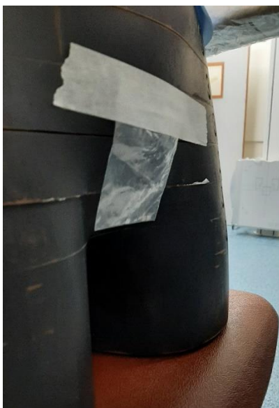
Figures 5 and 6. Demonstrating the location of the TLD placement into the left and right ovary positions of the anatomical holder (blue plate) of the phantoms pelvis.
