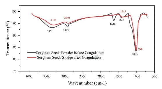
Figure 5. FTIR spectra of Sorghum seed powder (black line –) and sludge after treatment (red line –).
