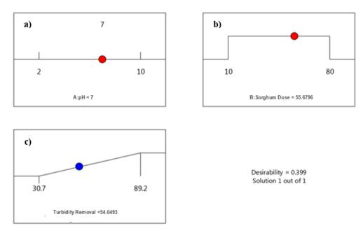
**Figure 4.** Optimization of treatment variables at pH range 7–8.5: (a) pH = 7; (b) dose = 55.7 mg/L; (c) turbidity removal = 54%. Red balls show the input variables while blue balls show the response value (turbidity removal efficiency).
