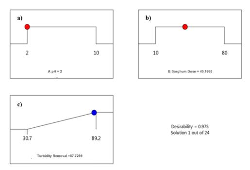
**Figure 3.** Optimization of treatment variables for Sorghum: (a) pH = 2; (b) dose = 40.2 mg/L; (c) turbidity removal = 87.73%. Red balls show the optimal input variables while blue balls show the optimal response (turbidity removal efficiency).
