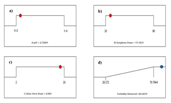
**Figure 9.** Optimization of treatment variables: (**a**) pH = 2.7; (**b**) Sorghum dose = 17.1 mg/L; (**c**) Aloe Vera dose = 0.9%; (**d**) turbidity removal = 84.2%. Red balls show the optimal input variables while blue balls show the optimal response (turbidity removal efficiency).
