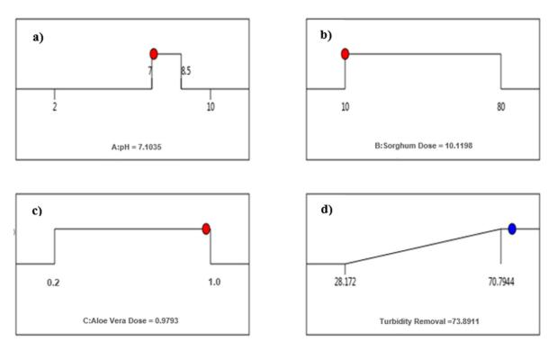
**Figure 10.** Optimization at pH range 7–8.5: (**a**) pH = 7.1; (**b**) Sorghum dose = 10.1 mg/L; (**c**) Aloe Vera dose = 0.98%; (**d**) turbidity removal = 73.9%. Red balls show the input variables while blue balls show the response value (turbidity removal efficiency).
