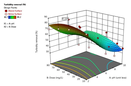
**Figure 2.** 3D response surface plot (Sorghum dose vs. pH) showing the performance (pH = 2; dose = 40 mg/L; turbidity removal = 87.73%; residual turbidity = 38.5 NTU).
