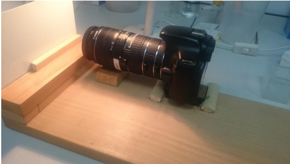
Figure 4.5. Photograph of rig setup for photography of individuals
