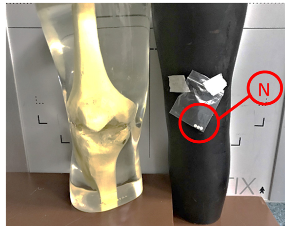
Fig. 4. TLDs 44 in batches of three positioned (N) as shown for ESD (absorbed) dose readings to the AP knee.
