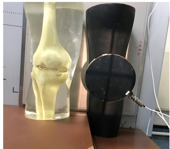
Fig. 2. Ion Chamber 37 positioning for AP skin entrance (absorbed) dose readings.
