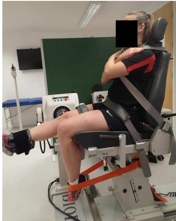
Figure 3.4 The setup position for all knee extension and flexion measurements
