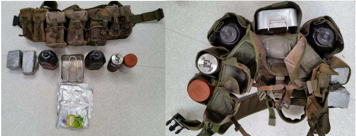
Figure 3.2 The webbing with external load, three water bottles were filled with water
