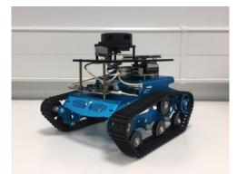
Fig. 1. Low-Cost Search and Rescue Robot Platform
