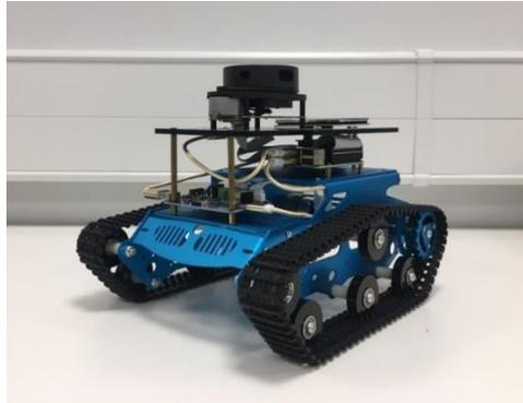
**Fig. 1.** Low-Cost Search and Rescue Robot Platform
