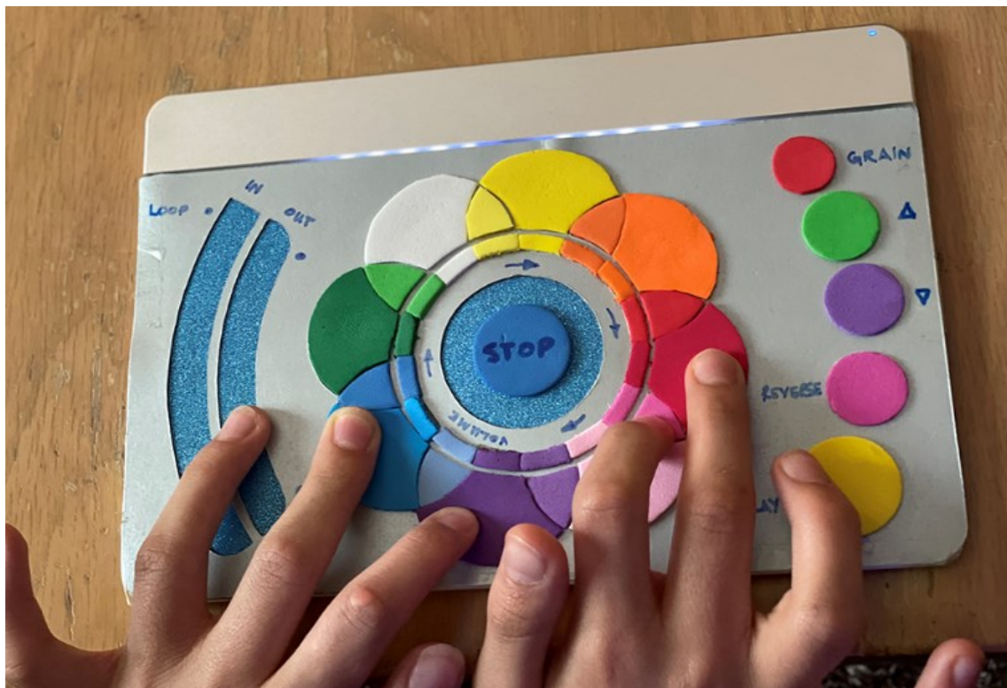
Figure 20. The floral multi-touch capacitive hardware interface.
