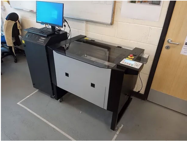
FIGURE 1. The intelligent computer-controlled cutting (ICNC) machine used to study the proposed cyber-physical system security for the manufacturing industry 4.0.
